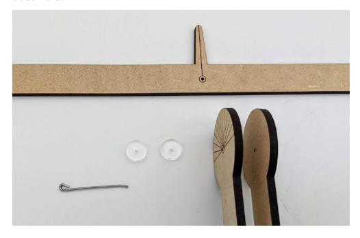
4. Slide the straight end of the paper clip through the two parallel holes in the top of the stand. It will pass through both washers and the hole in the center of the balance arm. Starting from the outside of the stand, the wire should pass through these layers in the following sequence: → stand → washer → balance arm → washer → stand→.
