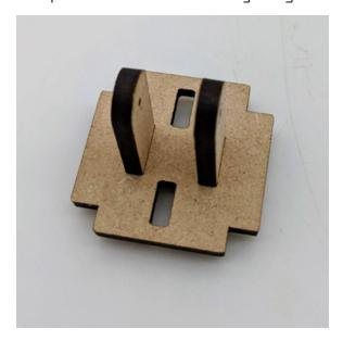
8. The two long curved pieces shown are connecting arms which attach the basket to the pivot. Lay out the connecting arms and the pivot base you just assembled in the same orientation shown.
