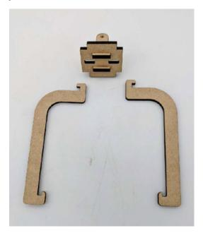
9. Insert the top ends of the connecting arms upwards into the two unoccupied slits in the pivot base. Push the ends of the connecting arms upwards as far as they will go, then gently slide each connecting arm outwards towards the edge of the pivot base. In this position, the notch in each connecting arm grips the pivot base to help secure them together.
