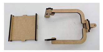
13. Once two basket sides are hooked onto the connecting arms, raise the pivot upright so that the basket sides align with the open edges of the basket. Push the sides together until the slots slip over the tabs to complete the basket assembly. Friction will hold it together quite well, but to attach the pieces even more securely, add a few drops of glue where the separate wooden pieces meet to reinforce the connection.
