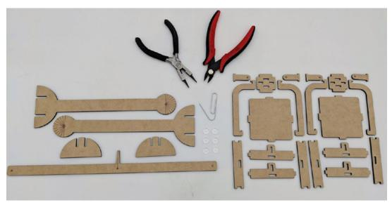
2. Construct the stand, which holds the balance arm. Take the two long wooden pieces with notched bottom edges and slot them into the two notched half-circles to assemble the stand.
