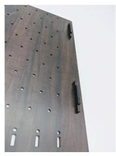
3. Insert the ten long pins into the base as shown. Each long pin contains "wings," which fit into two slots in the body piece. One wing fits in a slot at the bottom edge of the base and the other wing in a slot several inches above the first.
